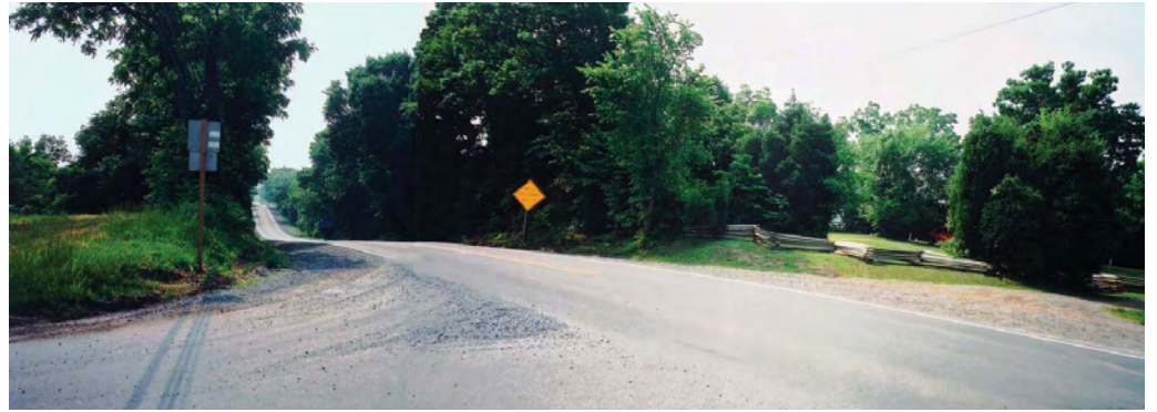
Traffic calming element should be introduced to improve safety at Watson Road, where limited sight distance is provided.
